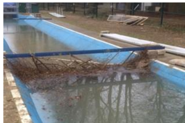
Fig 3: 0.45 m high wooden dam
